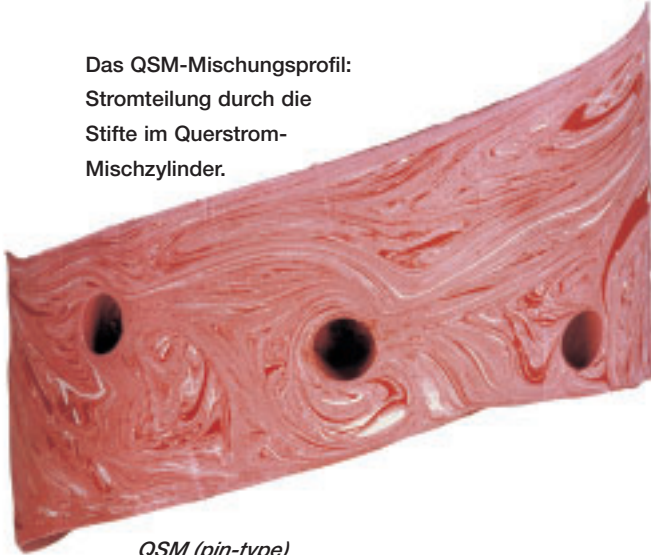
QSM (pin-type) compound cross section: flow division obtained by the pins of the pin- type mixing barrel.
